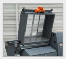
The grille and the enhanced vibrator ensure reliable, continuous material flow for an efficient pumping performance.
