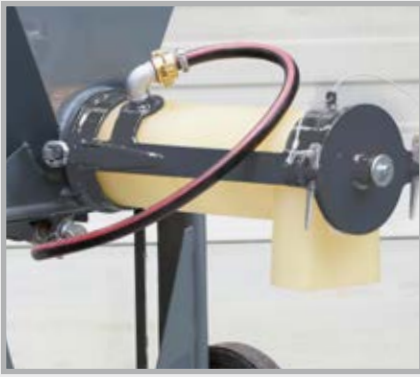
Rubber mixing pipe for rapid cleaning of the mixing zone
