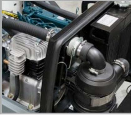
The extremely powerful 4-cylinder engine is exceptionally quiet due to the speed of only 2,600 rpm and extremely effective sound insulation.
